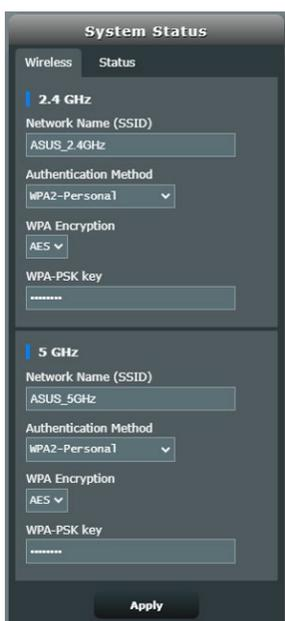
The screenshot shows the 'System Status' page with two tabs: 'Wireless' and 'Status'. Under the 'Wireless' tab, there are two sections for configuring security parameters for different frequency bands.
