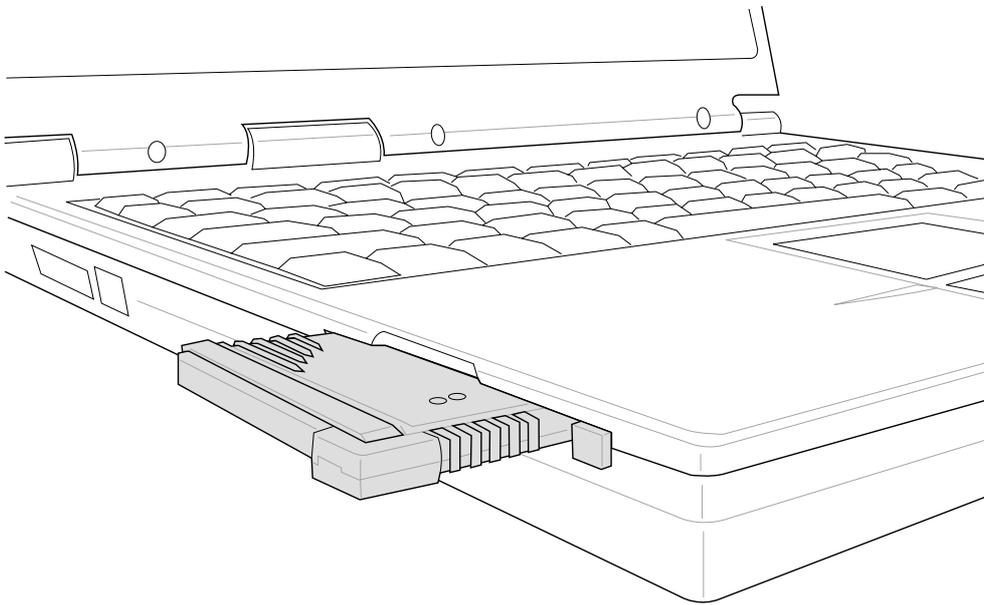
3. Windows will automatically detect the ASUS SpaceLink PC Card once it is inserted into the PCMCIA slot, then the “Add New Hardware Wizard” dialog will appear. Click **Next**.
