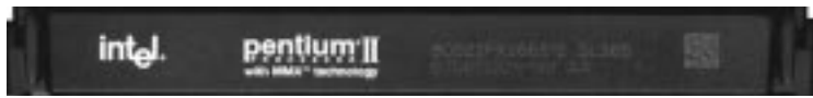
Intel Pentium II Processor in a SEC Cartridge (233-400MHz 512KB/128KB/0KB L2 Cache)
