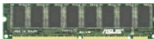
Non-ECC SDRAM DIMM (8 chips)
